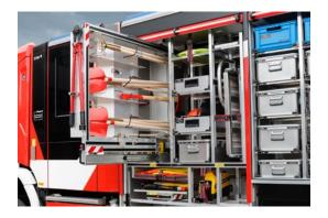
**Optimum use of every space** Pull-out equipment walls make it easier to remove equipment items and use space wisely.
