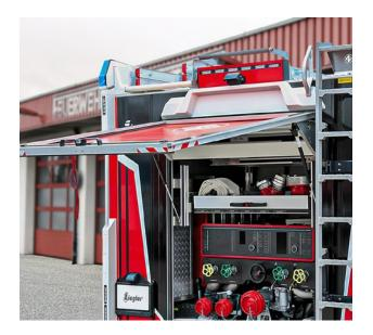
**Rear flap with integrated roller shutter** The rear flap serves as weather protection. Due to the integrated roller shutter, everything can be seen and coupled without restriction even in the narrow equipment shed.
