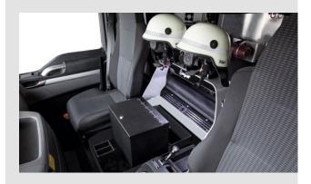
Document box and charging holders for handheld radios and lights can be placed in the free space between driver and co-driver. With putting the helmets on the holders with closed chin straps you already fix them in place. Developer, manufacturer, trader and service provider all from one source.
