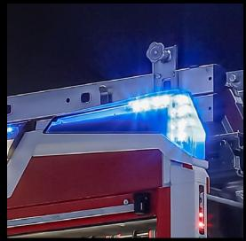
Tailfin beacon on the end of the superstructure Integrated into the corners of the superstructure, the Tailfin warns not only while driving, but also when using the access ladder or lowered ladder frame to the rear and sides.
