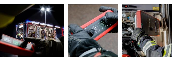
**Manual control unit for light mast control** Large buttons ensure safe and easy operation even when wearing gloves. The pneumatic light mast can be extended via the manual control unit. The powerful LED spotlights can be rotated up to 360° in the desired direction and tilted into two separate areas. **Swivel-mounted control panel** Easy accessibility of the components for inspections and emergency operation is ensured by a swivelmounted installation.
