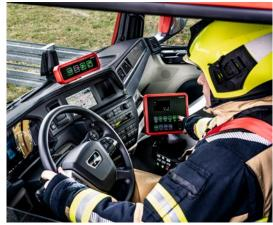
**Ergonomics and clarity in the cockpit** The machine operator and crew leader can easily overview and control all important functions via two separately arranged control panels.
