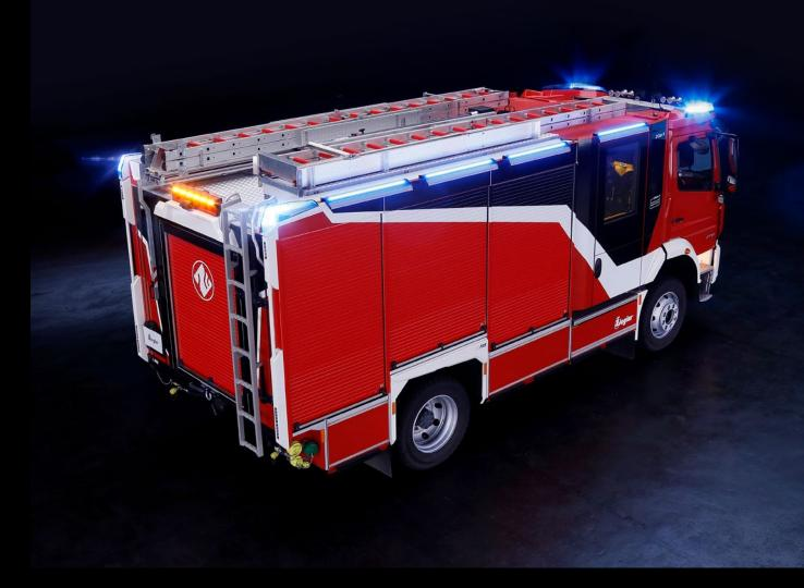
**Beacons on the side** Up to five LED blue light elements mounted on the side reinforce the rear beacon and thus guarantee the visibility of the vehicle in road traffic.
