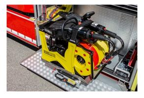
**Heavy equipment in the lower compartment** The hydraulic rescue kit is loaded in a way allowing quick and effortless removal.
