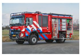
water supply. In addition, the vehicle has an ALCO APF 1DC 450 front turret with an output of up to 1,000 liters per minute and two roof turrets that can be controlled manually through the roof hatch.
